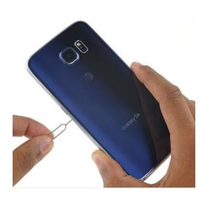
Tips: The back glass is thin and will need time and precision once it's already cracked it will continue to crack therefore let your customer know ahead of time if the back glass isn't the initial repair. Now, if the glass is not already cracked take your time with these steps. Tools: Philips screwdriver
