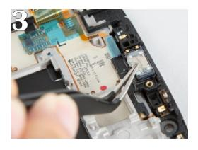
• Next, you will want to remove the ear speaker. New full assembly G5 parts come with the housing and lcd all together. Because of that the only the camera and ear speaker will need to be transferred over to the new assembly from the old.
