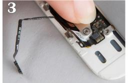
Tip: Make sure to lay metal bracket in properly with rounded edge on the bottom. Then screw down the flex cable. Not to tight on any of the screws if so, with the screws to tight on the plate the home button won't click it will feel stiff.
